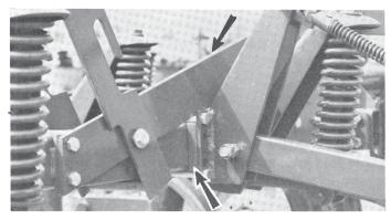
3a. The first mounting bracket on each wing is located under a brace and needs special spacers (see arrow) and longer bolts for mounting. Summers JD1510 Chisel Plow mounting package (PN 8H1590) includes 8 spacer plates and 16 - 5/8 x 7" bolts. Spacer plates are also supplied for use on the outer mounting bracket on each wing so sections run perfectly square.
